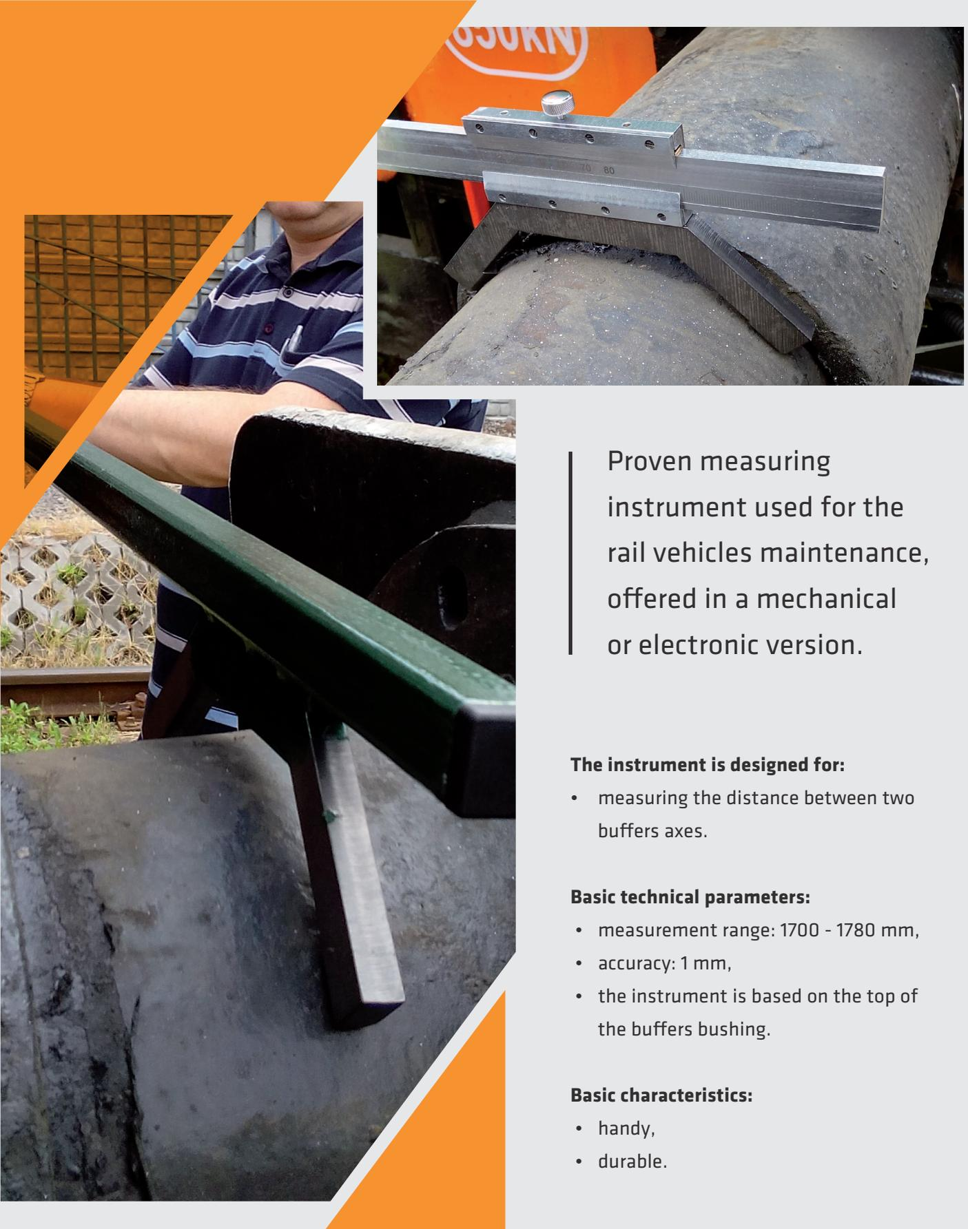
Proven measuring instrument used for the rail vehicles maintenance, offered in a mechanical or electronic version.
